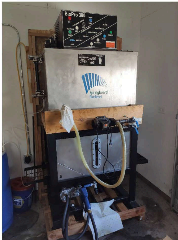
Photo 23: A view of the BioPro 380 from Springboard Biodiesel. This machine has some old biodiesel in it that will need to be drained and disposed of. The machine can then be cleaned in order to be sold by LTBB.
