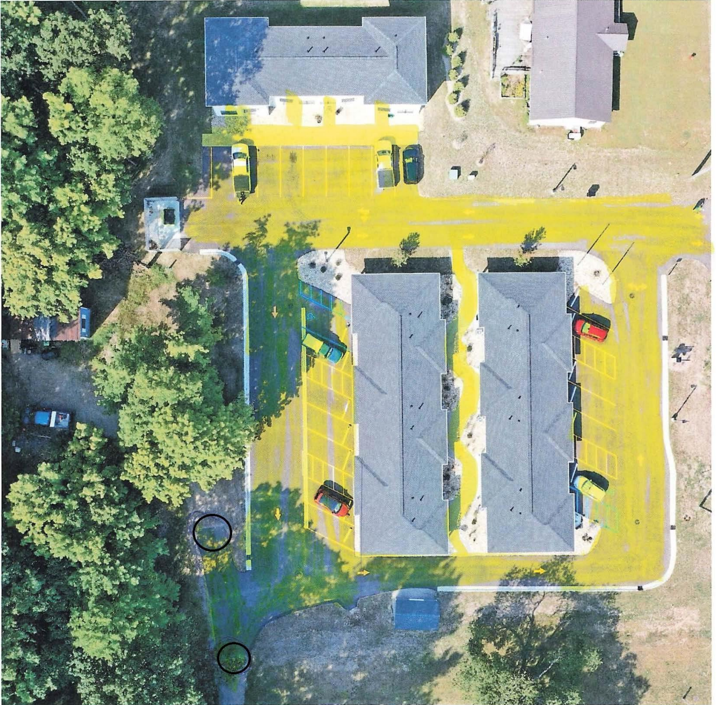
Exhibit 1 Area in Yellow to be plowed Area circled in Black must be kept clear
