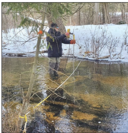
Water Quality staff collecting discharge (amount of water moving past a point per second) on Big Sucker Creek.
