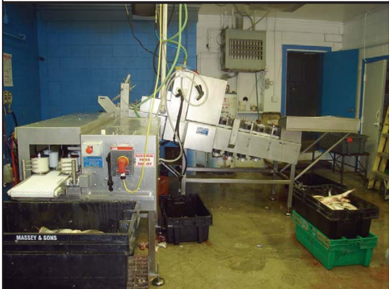
Bell's Fishery bought the file machine AHF 225 from Pisces UMK Inc. in October. The machine filets 43 fish a minute. Photo by Annette VanDeCar.
